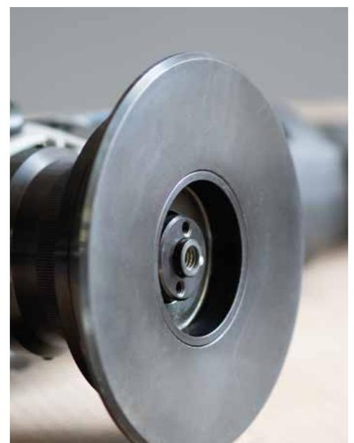
The Bevel Mate® concept works 50% faster and considerably quieter than with a sanding disc and without grinding dust. The end result is exact in radius and without burrs, so no post-processing is required.
